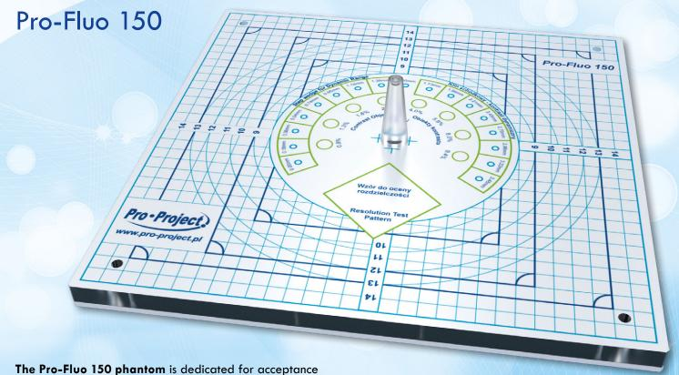
and constancy tests of radiography and fluoroscopy equipment according to the new DIN 6868-150 standard.
